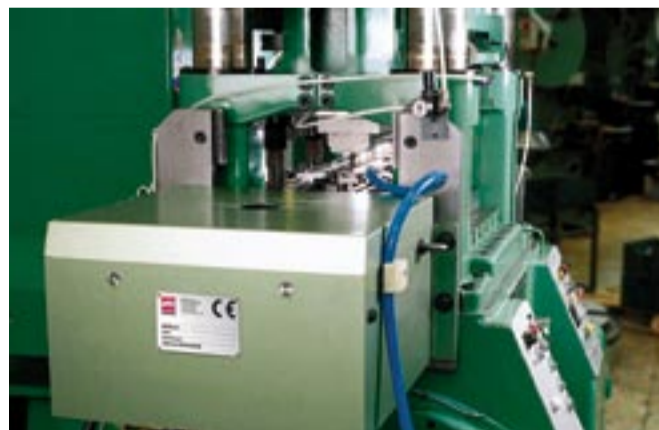
DIGIEMME mechanical transfer on BRUDERER Press BSTA 60
