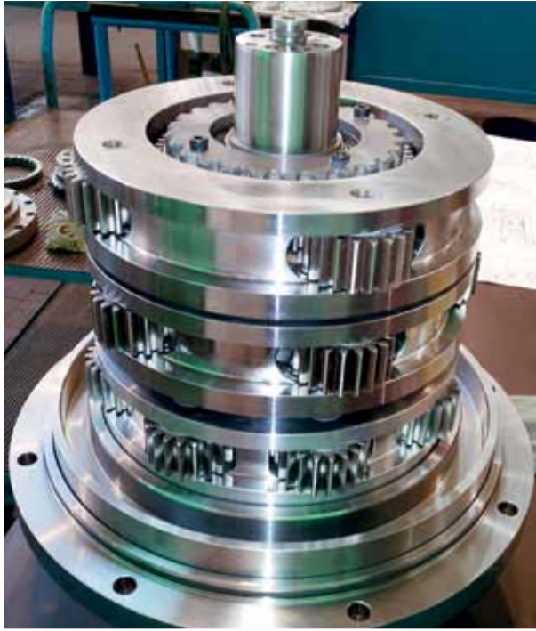
The three-level planetary gearbox
