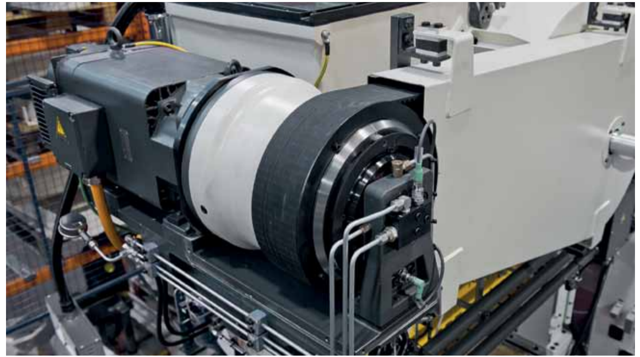
A planetary gearbox with all connection lines mounted on the main motor
