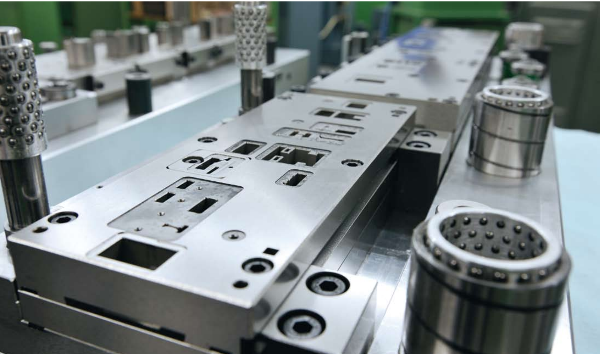
In the future, tools will be made a little larger at Zetka thanks to the extended bed width of 1250 mm on the new BSTA 510-125. The punching press guide system is also ideally situated along same die line level as that of the press tool.
