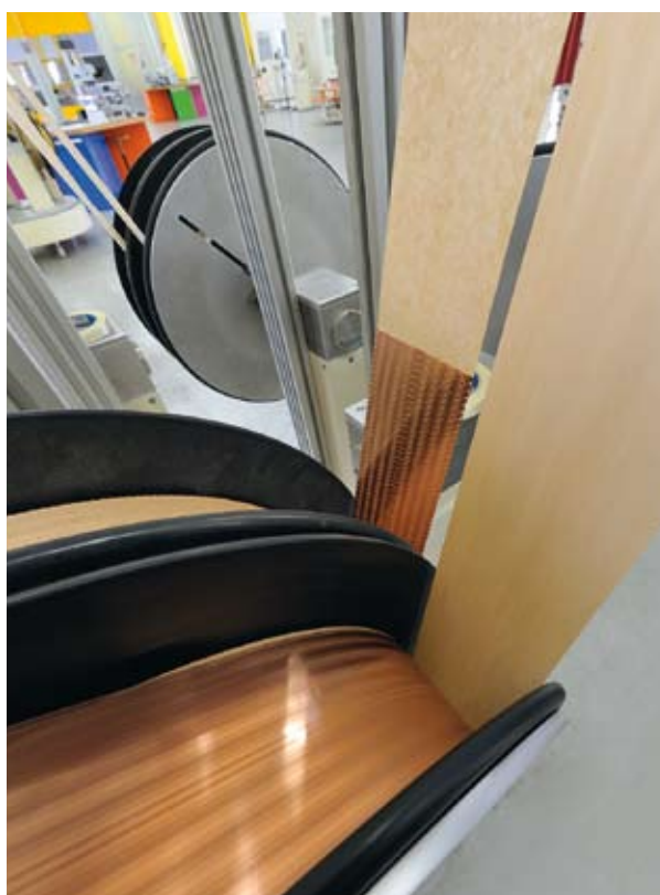
Coils are wound automatically.
