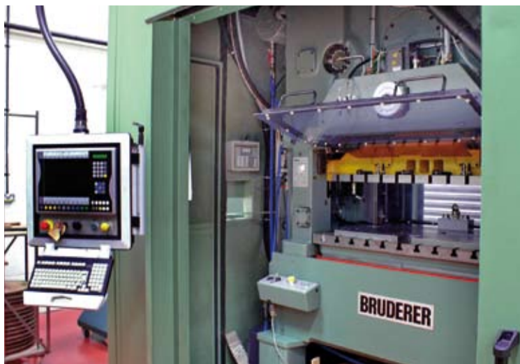
The newest Bruderer punching press installed in Cirencester is a long-bed machine from the BSTA 300-85B series.
