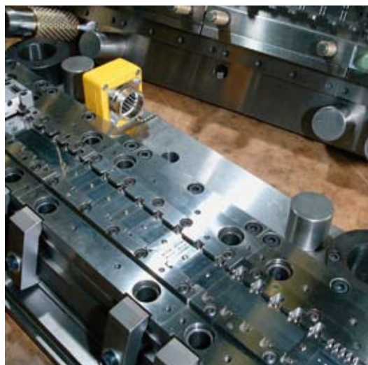
Multi-station multi-out die as used at Batten & Allen on Bruderer automatic punching presses.
