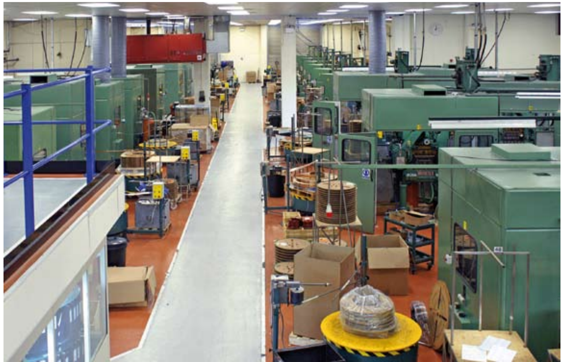
Manufacturing at Batten & Allen in Cirencester: Predominantly dies from internal die and mould construction are used on 24 Bruderer high-speed automatic punching presses. Every eighth employee performs testing functions on a random sample basis.
