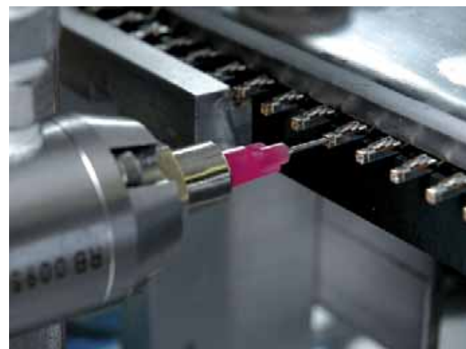
Inserting of gel to contacts for the automotive industry
