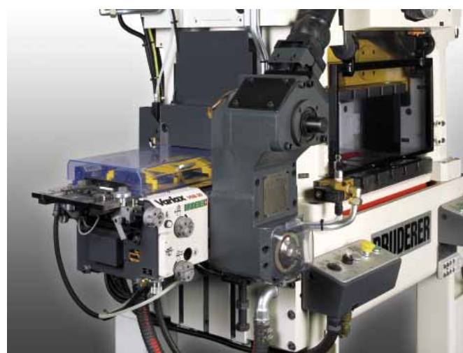
Gripper feeder type VGB 30 attached to a high performance stamping press BSTA 250
