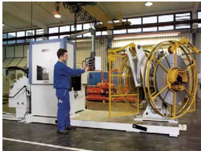
High-precision leveller/straightener combined with double end decoiler for optimum levelling/straightening results and high availability
