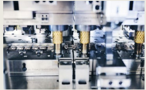
Step 1 The material for the plug contacts is stamped and formed as required.
