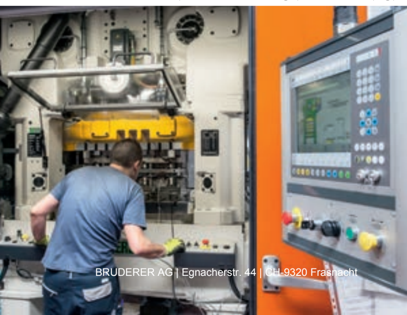
3-shift operation: BSTA 810-145 high-performance stamping press.
